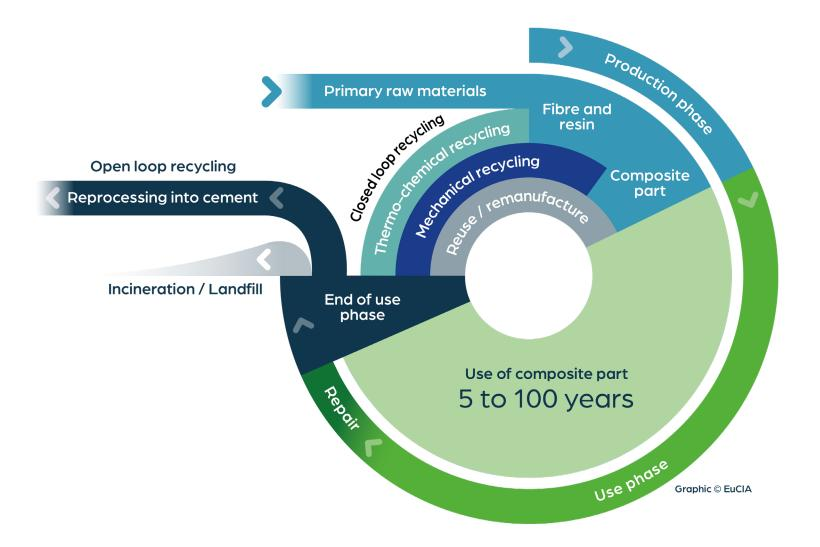
Cement co-processing is both commercially and technically proven for treating end-of-life glass reinforced composite materials and can immediately be deployed at large scale
